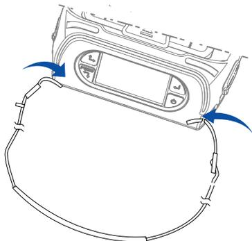
Insert the strap into the hook of the printer.
