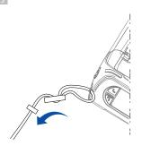
After pulling out the end of the strap tightly, put it into the clip to be fastened.
