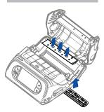
Assemble two (inner & outer) External Paper Guides as shown in figure and press three points to fix firmly inner guide with outer guide.
