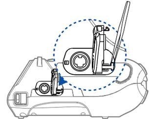
Using a sharp tool, insert the Cap Hook to the hole which is located in the right side of Interface Cap.
