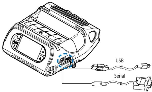
1. Connect the USB or Serial cable to the cable connector on the printer.
