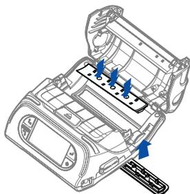
Assemble two (inner & outer) External Paper Guides as shown in figure and press three points to fix firmly inner guide with outer guide.
