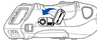
When Cap Hook inserted, install the Cap Cover in direction of an arrow as shown in the image.
