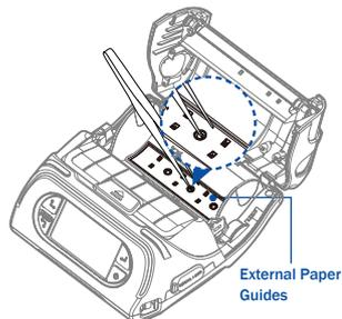
Using sharp tool, push External Paper Guides in order to detach from the printer. Press circle on the middle of external paper guide with tool.
