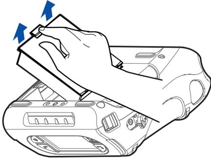
Remove the battery. Lift out the battery.
