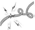
Do not bend the wire and do not allow the wire to be pressed by heavy object.
