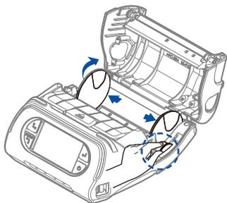
Open the Paper cover by pressing the Open button and set the width of paper guide by turning the knob with finger.
