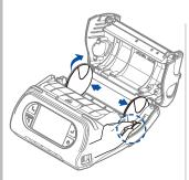
Open the Paper cover by pressing the Open button and set the width of paper guide by turning the knob with finger.
