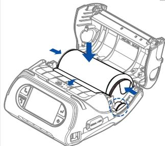
After inserting the paper, adjust the paper guide to little wider than paper size. Then pull the paper out and close the paper cover.
