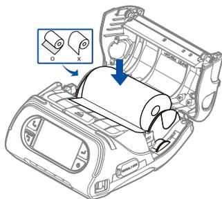
Put the stock in so it unrolls from the bottom. Remove the stock core when it is empty. Pull a short length of stock out of the printer.
