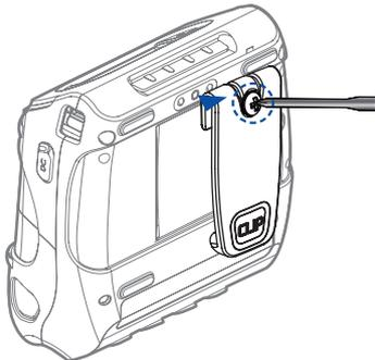
Tighten the screw with driver as shown.
