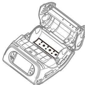
Two external paper guides will be installed to printer.
