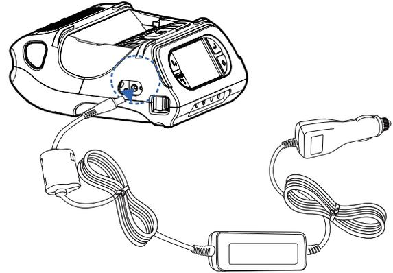
Connect the vehicle charger to the printer.
