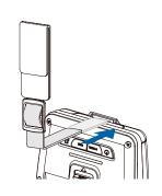
Put the strap into the strap bracket hole as shown.
