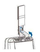
Turn the strap and printer over and put the strap into the hook as shown.
