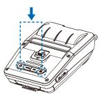
While you are holding the FEED button, press the power button.
